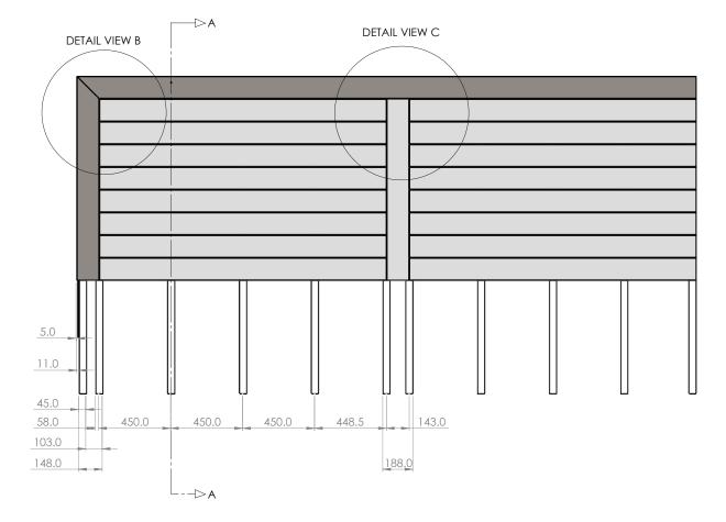
Plan View showing typical timber joist layout, decking board and edge board detail:
