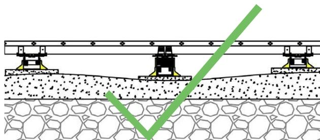
NewTechWood products can be stored on pedestals or jacks if the surface is uneven, as shown above. Consult with the pedestal or jack manufacturer before using the product to ensure its compatibility with NewTechWood's products.
