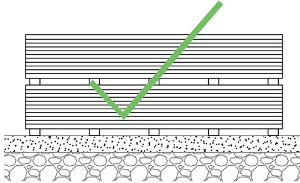
NewTechWood products shown above put on a flat surface on joists is the correct way for storage.
