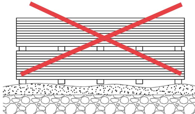
NewTechWood products stored on an uneven surface will make the products prone to warping and distortion.
